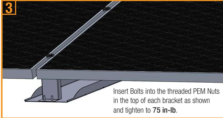
Insert Bolts into the threaded PEM Nuts in the top of each bracket as shown and tighten to **75 in-lb.**
