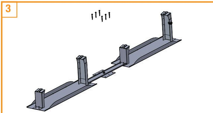
Replace the connect belt on the system and secure the 1/4-20 Serrated Hex Flange Nuts to **75 in-lb.**
