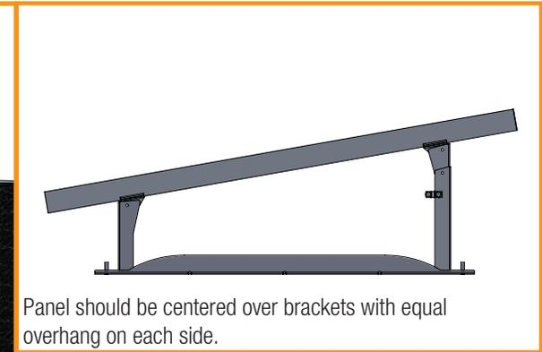
Panel should be centered over brackets with equal overhang on each side.
