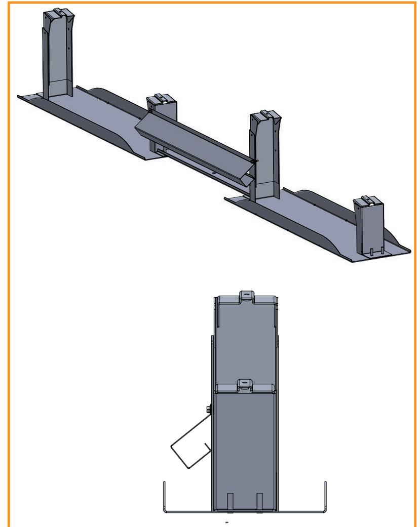
The Wire Management Raceway can be used to run conduit and wires both through an array and from one array to another.
