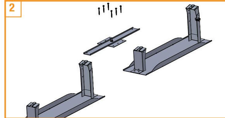
Tighten 3/8 Serrated Hex Flange Nut to **200 in-lb.**
