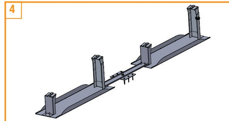
Insert 6 x roof appropriate fasteners through the holes in the SAP.
