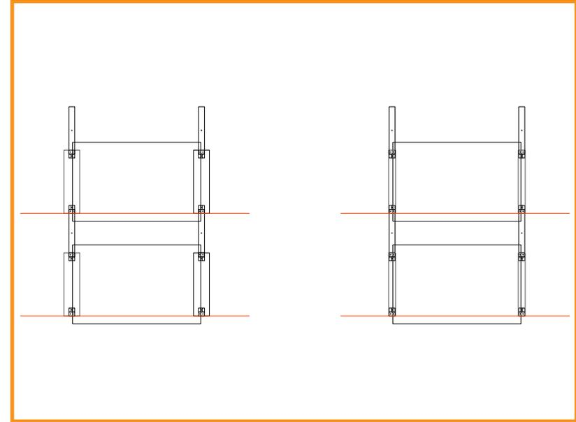
Horizontal chalk lines will mark placement of the short edge of the ballast pan (or Solar Belt). When planning a layout, leave correct spacing from the edge of the ballast pan (or Solar Belt) to the edge of the panel to avoid encroaching into the fire walkways (about 4" for typical 60 or 72 cell panel).
