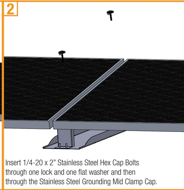
Insert 1/4-20 x 2" Stainless Steel Hex Cap Bolts through one lock and one flat washer and then through the Stainless Steel Grounding Mid Clamp Cap.
