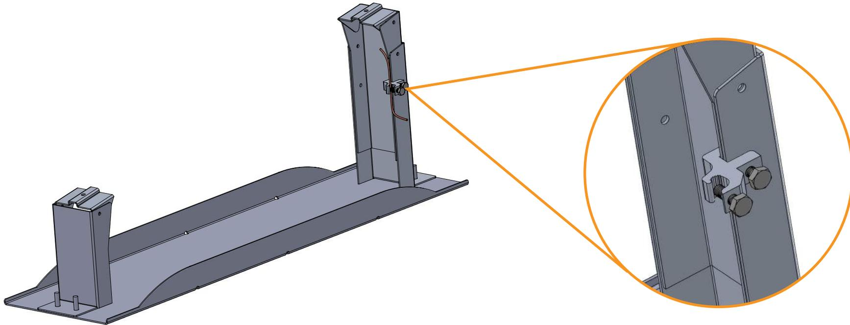
Ground lugs should be placed before PV Modules are installed. As a general rule, one SGB-5 Lug is required for every 56 modules in array. Apply lug to the edge of a high or low bracket as shown above. Bolt should be torqued to 20 in-lb.
