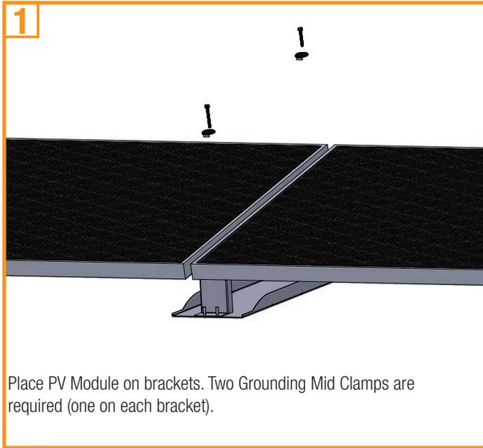
Place PV Module on brackets. Two Grounding Mid Clamps are required (one on each bracket).
