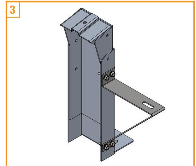
The Accessory Mounting Plate (AMP) should be attached to either side of the High Bracket using up to 4 x #10 Stainless Steel Self Tapping Sheet Metal Screws. When choosing a position on the bracket, make sure that placement of ballast blocks or panels won't interfere with the attachment or the accessories being mounted to the attachment.
