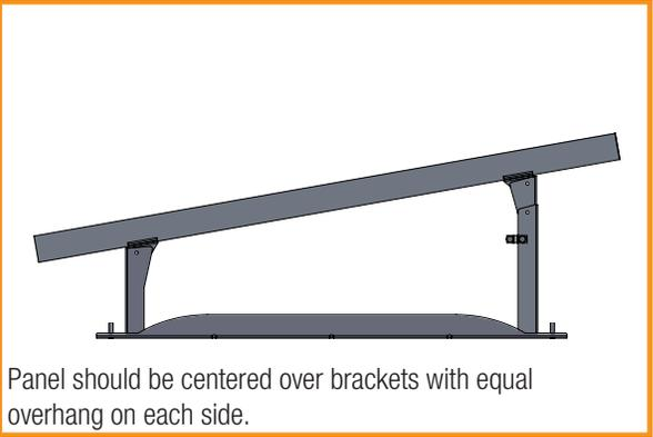
Panel should be centered over brackets with equal overhang on each side.
