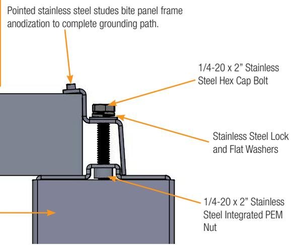
Pointed stainless steel studs bite panel frame anodization to complete grounding path.
