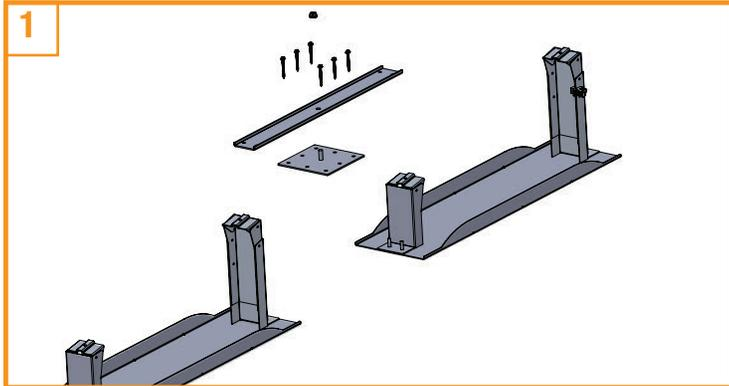
The Seismic Attachment Plate (SAP) is connected to the system through the center hole of the Connect Belt. Not every Connect Belt will need an SAP. Consult a qualified structural engineer to determine quantity and placement of SAPs.
