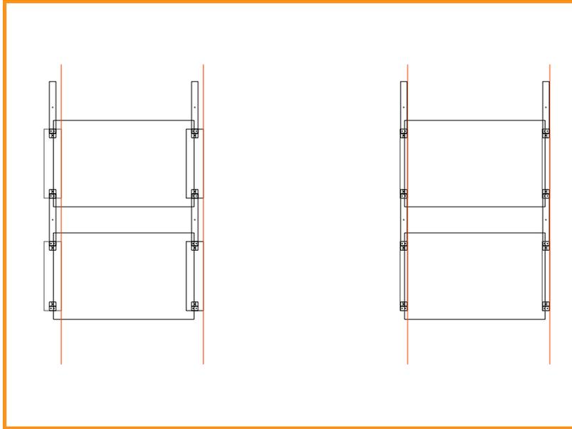
Vertical chalk lines will mark placement of the long edge of the ballast pan (or Solar Belt). When planning a layout, leave correct spacing from the edge of the panel to the edge of the ballast pan (or Solar Belt) to avoid encroaching into the fire walkways.
