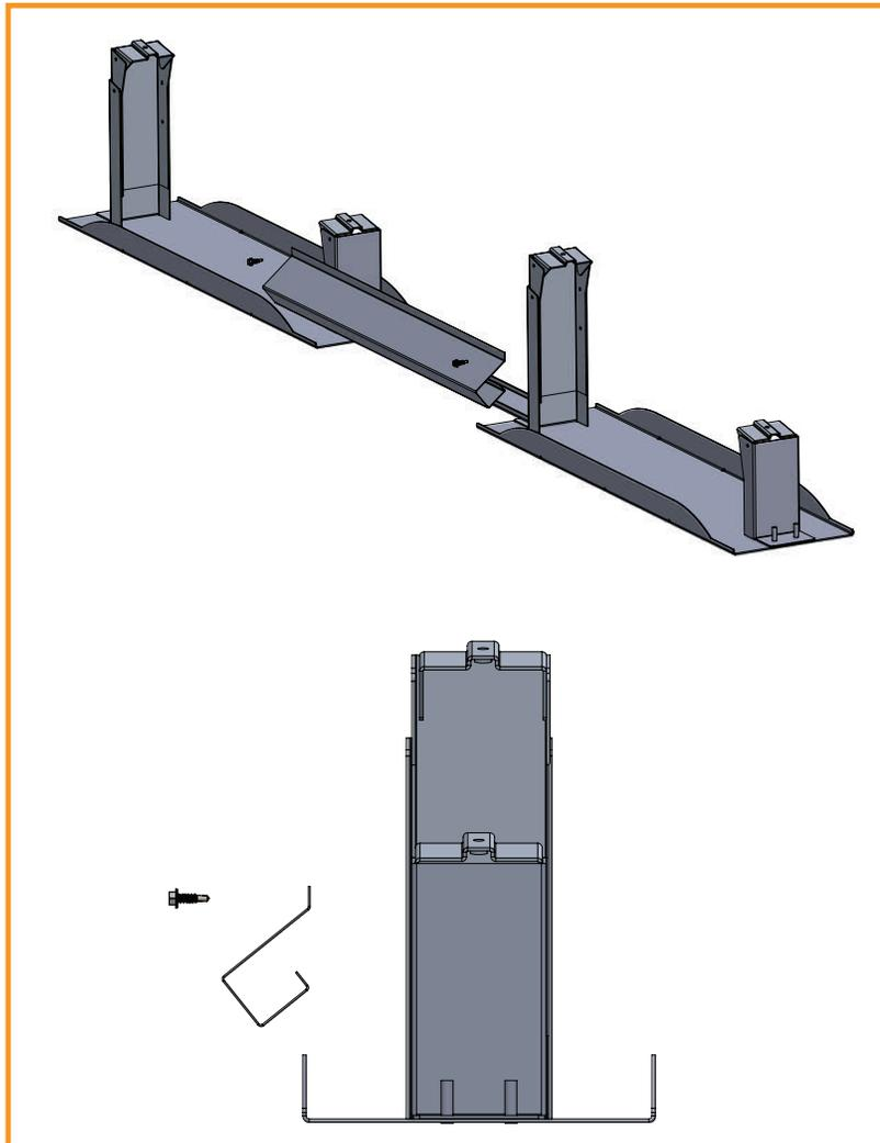
The Wire Management Raceway should be attached to the sides or back of the High Bracket or Low Bracket using #10 Stainless Steel Self Tapping Sheet Metal Screws. When choosing a position on the bracket, make sure that placement of ballast blocks or panels wont interfere with the attachment.
