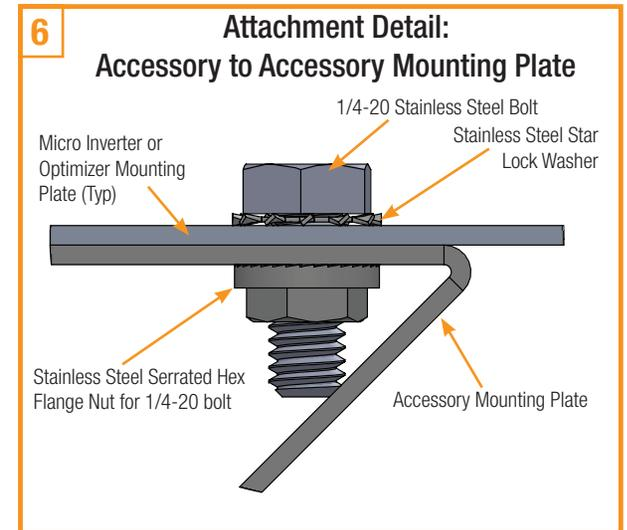
To attach an accessory to the AMP, use a 1/4-20 Stainless Steel Bolt with a Stainless Steel Star Lock Washer and a Stainless Steel Serrated Hex Flange Nut. Attach the accessory using the slot on the top of the AMP. tighten bolt to **65 in-lb**.
